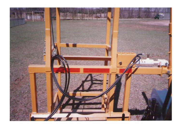
Before installation, review the picture above for the proper hydraulic hose connection. The looping of the hoses is very important when cage is lowered for loading.
