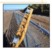
Stretching barbed wire or tension wire can be a time consuming job. With the Barbed Wire Dispenser from L&C Enterprises-USA, Inc. all three strands of barbed wire and two strands of tension wire can be put in place in half the time. The Barbed Wire Dispenser makes dispensing wire safer and faster.
