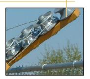
Stretching barbed wire or tension wire can be a time consuming job. With the Barbed Wire Dispenser from L&C Enterprises-USA, Inc. all three strands of barbed wire and two strands of tension wire can be put in place in half the time. The Barbed Wire Dispenser makes dispensing wire safer and faster.
