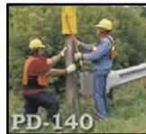
The **PD-140 Post Driver** is the perfect choice for driving Beams, Round, Square or Rectangular Tubing, Wood Posts, Stakes or any shape up to 4 inches.
