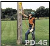
The **PD-45 Post Driver** can be operated by one worker and is the perfect choice for driving ground rods and various types of steel posts.
