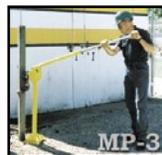
The Model **MP-3 Post Puller** weighs only 39.54 lbs (17.94 kg) and is easily operated by one worker.
