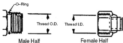
**How connection works:** This connection seals with an O-Ring on the male against a flat surface.
