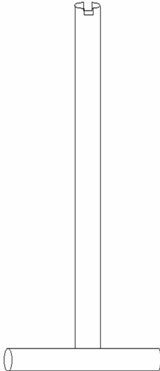
Extension for 8' Fence is made from 1 5/8" Tubing. A notch will have to be cut to hold the hanger from turning. See above. You can put a tee handle on the bottom
