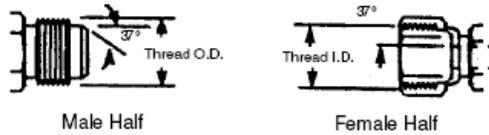
**How connection works:** This connection seals on two-mating 37° seats.
