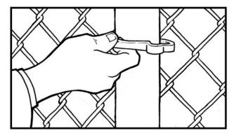
1. Place band around post and fabric, hook end in hand. Band requires no bending.
