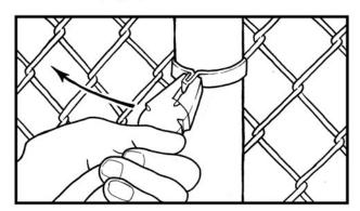
5. Turn closed hook toward post. Pliers may be parallel to post as shown or at right angles - erector's choice.
