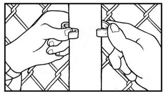
2. Bring ends of band together using pressure of thumb on hook end.
