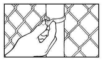
3. Place hook end over other end. Band can be held closed by light pressure at base of hook.
