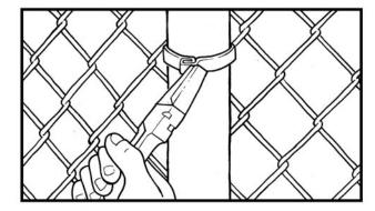
Use pliers to hammer hook flat against post. Over hammering will loosen band.
