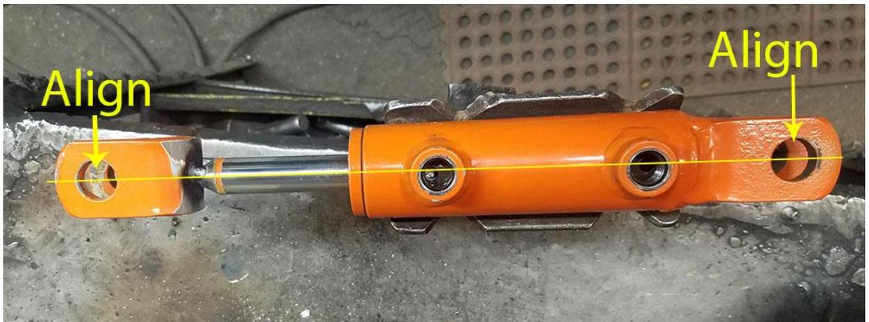
4. **Welding:** It would be preferred to weld using GMAW (MIG) indoors. A minimum of 26 Volts and a wire feed speed of 375 inches per minute will give proper heat-input. If welding with SMAW (Stick), try to maintain a minimum of 250 amps. Weld until the chamfer is completely full. Then, add a 3/16" fillet around the rod and clevis.
