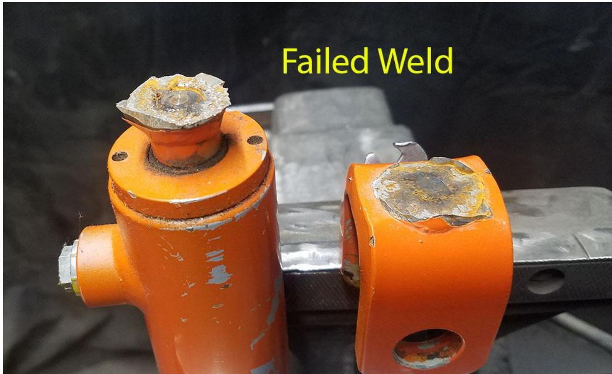
To improve the design of our cylinder and add more safety factor moving forward, we have modified the weld. The revised weld joint offers higher strength, as well as more joint access for our welders, which means less room for error.
